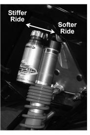
**WARNING!** Changing shock valving requires special tools and a sound knowledge of mechanical theory, tool use, and shop procedures to perform the work safely and correctly. Shocks contain high-pressure nitrogen gas. Use extreme caution when handling high-pressure service equipment. We recommend that this work be performed by a Polaris dealer.
